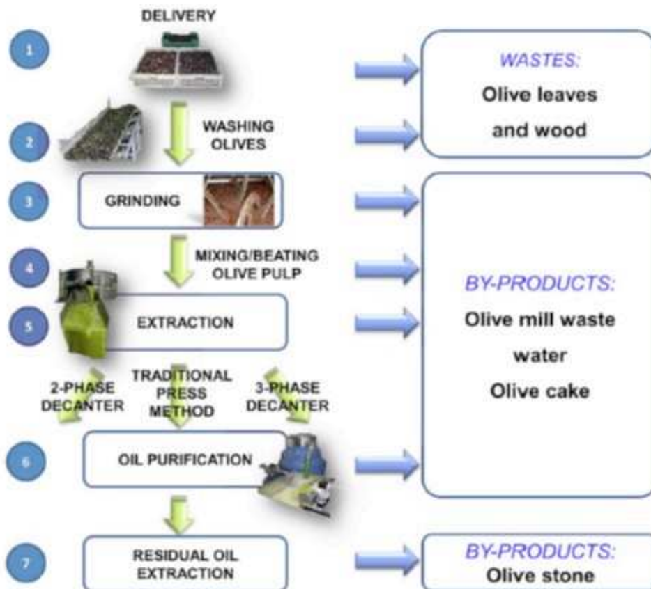
Figure 16.1: Wastes and by-products generated during olive oil production process (Roselló-Soto et al., 2015).
